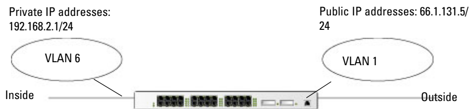
Figure 4 Example: Source NAT using Controller IP Address
